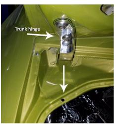
2) Locate and mark a spot in the center of the weather strip channel, directly across from the center of the trunk hinge as shown. Drill ¼" hole at the mark.
