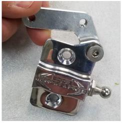
1) Apply anti-seize to the 1/4" X 3/4" socket cap flathead bolt and loosely fasten the "L" bracket into the hole in the outer corner of the Upper Strut Mount as shown.
